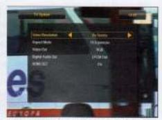
Thanks to its 'by source' option, the Ariva can output video at the resolution of the broadcast. That way, you can rely on the TV's inbuilt scaler
